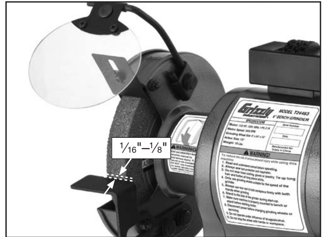
Figure 12. Model T24463 tool rest gap.
